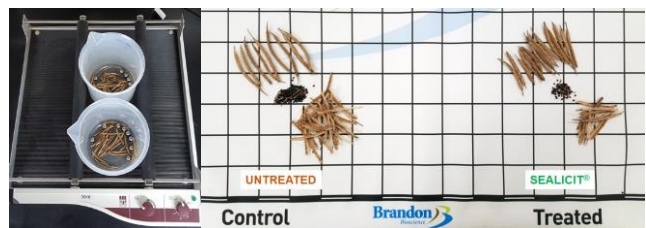
Random Impact Tests: untreated pods shed more seed in a given time under stress vs. SEALICIT treated pods
