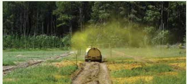
FIG 2. 2.9M/SEC WIND AIR INCLUSION NOZZLES + DRIFTSTOP
