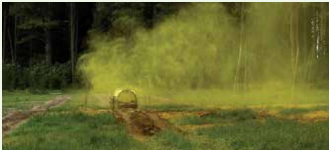
FIG 1. 3.5M/SEC WIND STANDARD SPRAYING SYSTEM NOZZLES + LATRON B
